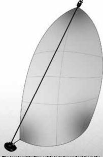
The torsional furling cable is independent from the spinnaker. The sail starts furling from the top and finishes at the tack, aptly named "top-down furler".
